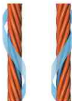
S-Lay (counter-clockwise, left-hand direction)
