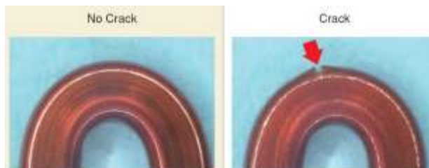
Image of the flexibility test «Coating Cracking»
