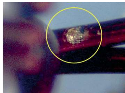
Scratches and peeling of the varnish on the wire coating
