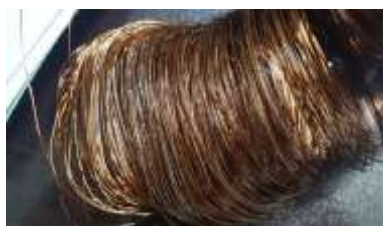
The presence of bubbles and burns on the Enamel wire
