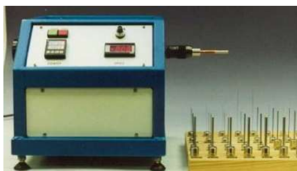
MANDREL WINDING TESTER STANDARDS: IEC 60851-3.5, JIS C 3216-3, NEMA MW 1000
